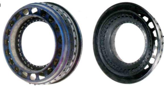
FRONT AND REAR VIEW OF AN ANNULAR, OR RING, COMBUSTOR FROM A NEW GENERATION ENGINE. Photos Courtesy CFMI
